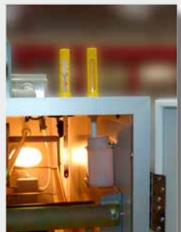
Thermo-hygrometer kit for temperature and humidity reading.
